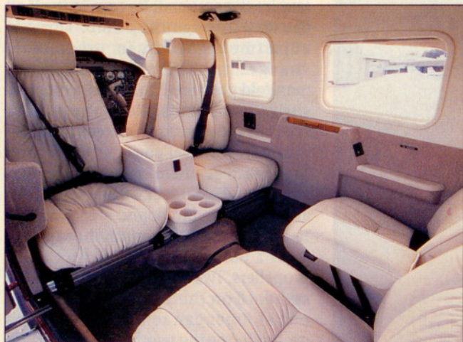
Piper still offers a six-place interior for the Seneca V (below), but the standard airplane comes with five seats and an Executive Console (above and above, right). Dedicated doors allow easy access to the aft (right) and nose baggage compartment.
